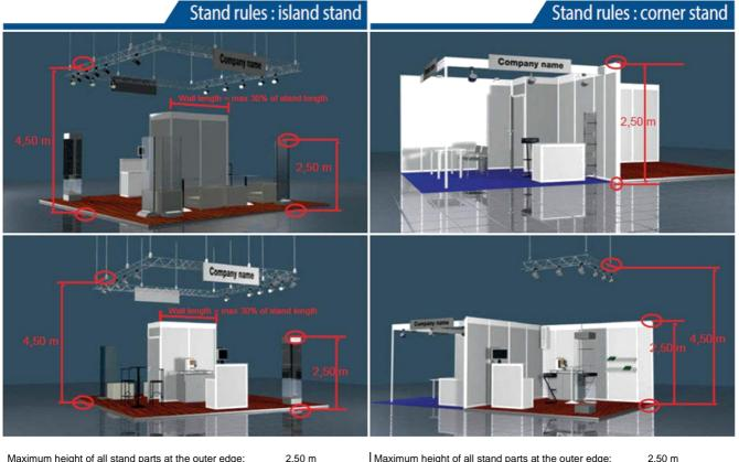
Maximum height of all stand parts at the outer edge: 2,50 m Maximum height of all stand parts in the stand: 4,50 m permission by ERS is required Unbranded rigging: 6 m
